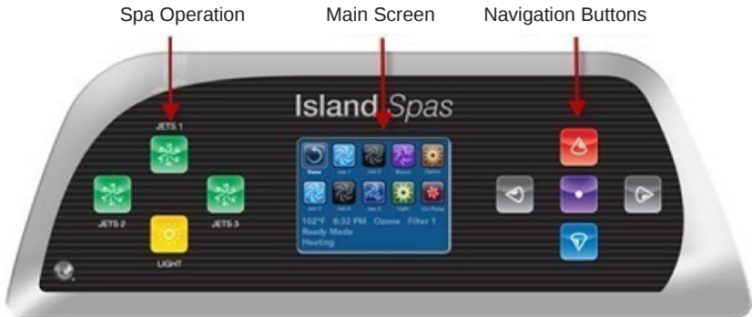
Island Spas 3 Pump Topside
