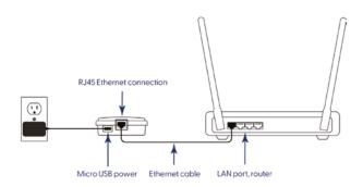
To allow communication between the CO and EN module, the EN module needs to be installed on a router.
