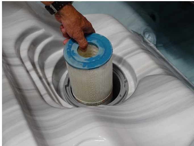
Figure 16. Drop in filter removal
